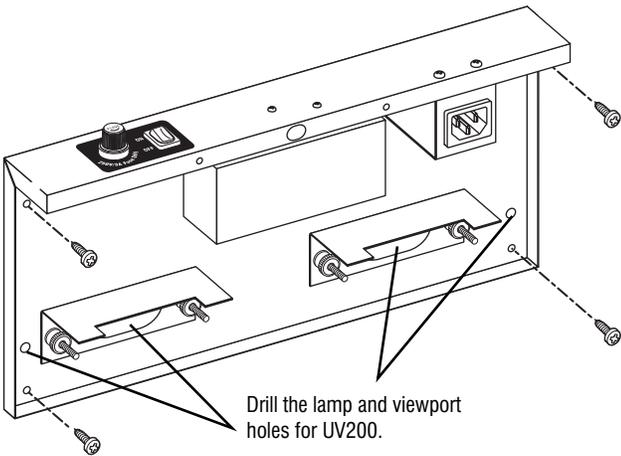
**Fig. 5** Mount the device using included sheet metal screws.
